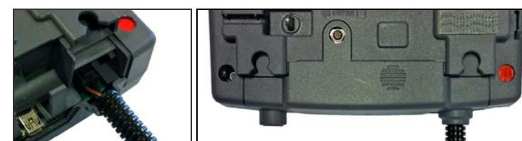
**Tip:** It is not necessary to seal the screw on the OBU's battery compartment cover covering the power connector, as specified by Satellic at [www.satellic.be](http://www.satellic.be).
